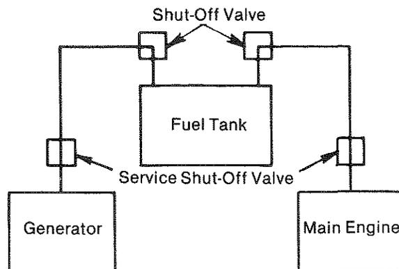
Fuel lines should be routed and supported to prevent leaks from vibration and chaffing. The line should be supported every 12 - 14 inches. Use as few connections as possible.
