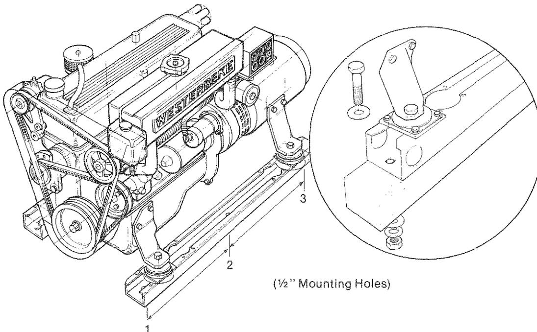
Three 1/2 inch bolt holes are in each generator mounting rail to be used in properly securing the generator to its mounting platform. These holes are on 15 inch mounting centers.
