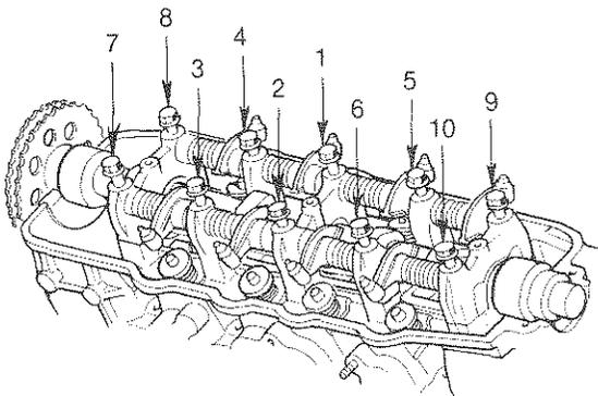
Head bolt tightening torque:
