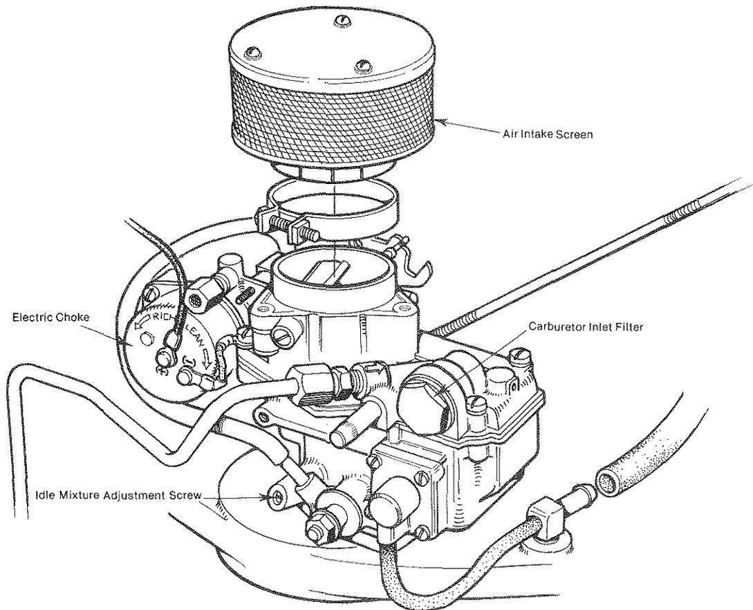
**NOTE:** Choke index mark is located on the choke cover lower right inboard side.
