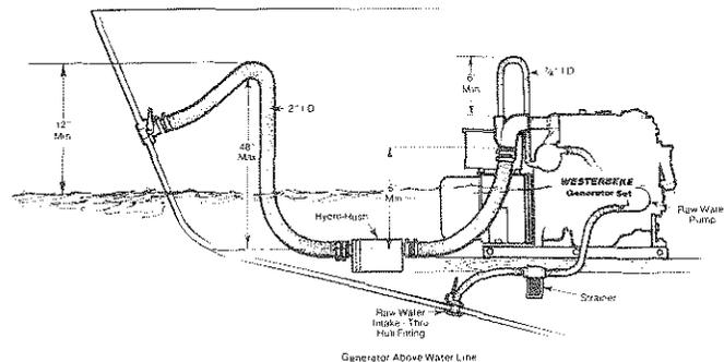
(e) Hydro hush mufflers should be mounted as close to the generator as possible and the exhaust/cooling water mixture from the exhaust injected elbow should drop down into the muffler.
